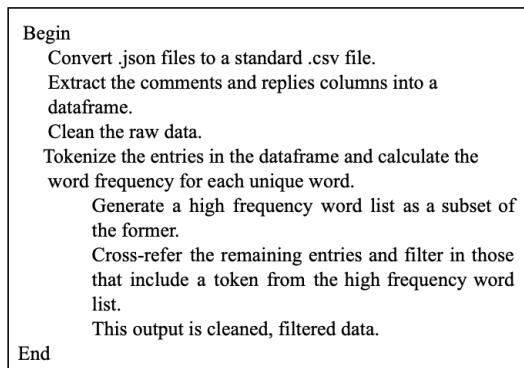
Figure 6: Algorithm Comment filtering
