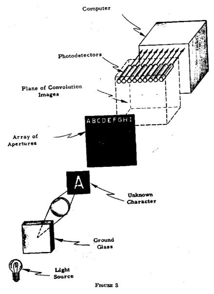
The light passing through, or reflected from, the unknown transparent character then diverges and passes through the array of standard apertures, and thence to a corresponding array of photodetectors. The electrical outputs from each of these detectors are ultimately processed and fed to the translator or to a recording tape for ultimate use with the translator.
