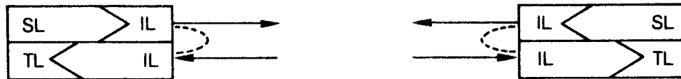
Fig. II-3b. Two-way terminal, which also permits generation of text in one's own language, in such a way that others can receive it in their's. The dashed arc indicates the possibility of a loop-test.
